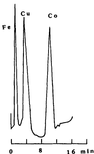
Figure 10. 4 nmole Fe, 2 nmole Cu, 1 nmole Co by quenching detection. Wescan HS column (150 X 4.2 nm), 0.2 M K-citrate 0.5 mL/min. PCR: 100 \mu M Al, 300 \mu M HQS, 500 \mu M HTA-chloride, 0.3 M MOPSO pH 7.9; effluent pH - 7. 610 V, 100 nA FS.
